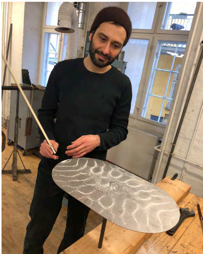
Building and testing the Chladni Plate, a device that reveals vibrational patterns of sound
